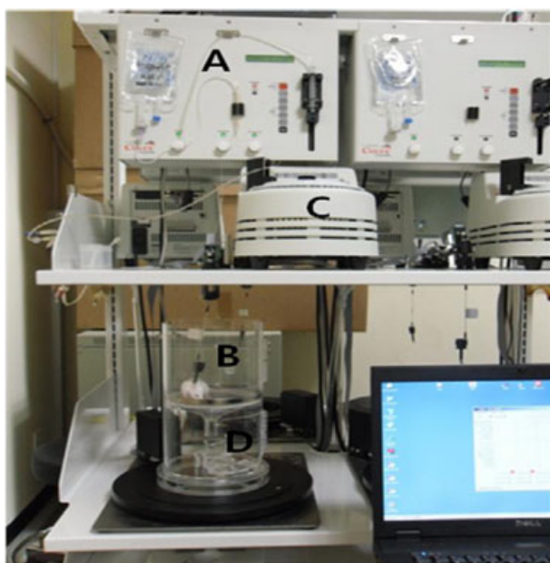
Figure 2. Automated blood sampling unit consisted of an automated blood sampler (A), fraction collector (B), freely moving mouse containment device return (C) and urine collector (D).
